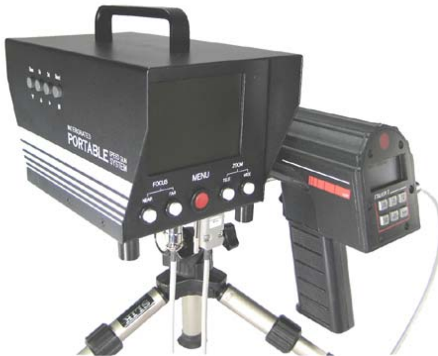
Figure 65: Integrated Portable Speed Gun System Interface with Radar Gun (Stalker II SDR)
